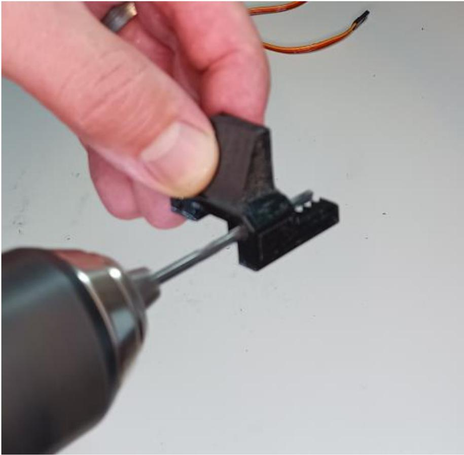
Use 3.1mm drill bit to clear both rail holes in the 3D printed jaw1 and jaw2 parts.
