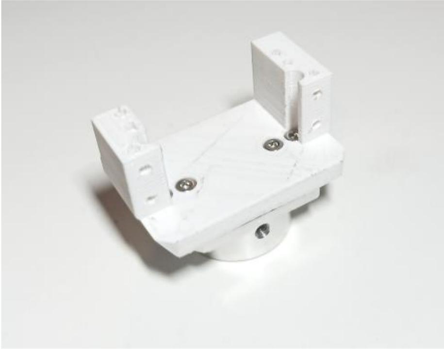
Use (4) M3x10 cap screws and M3 nyloc nuts to secure base to J6 mounting flange.
