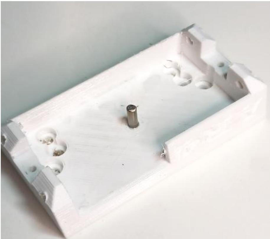
Insert glued end into carriage center hole and tap down into place. Shaft need to be fully inserted flush to bottom surface of carriage.
