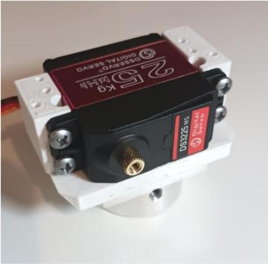
Secure servo to base assembly as shown and secure with (4) #6 screws
