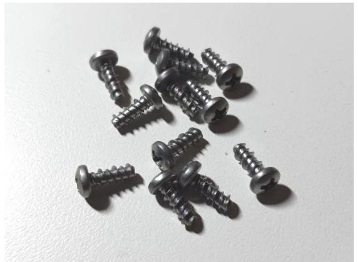
(12) #6 x .375 or equivalent round head screw. I prefer thread forming screws for use with 3D printed components but any screw can be used.
