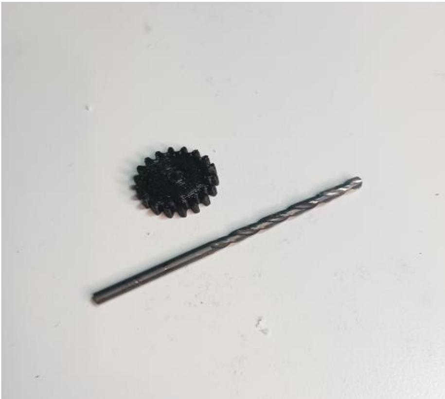
Use 3.1mm drill bit to clear center hole in 3D printed gear.
