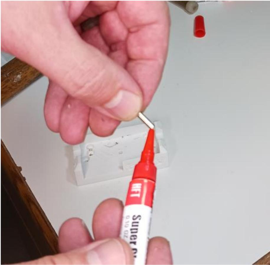
Place small drop of super glue on end of 16.5mm long shaft
